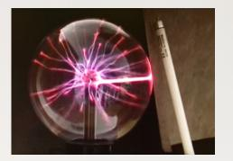
The fluorescent tube goes out as soon as the material is placed in between.
